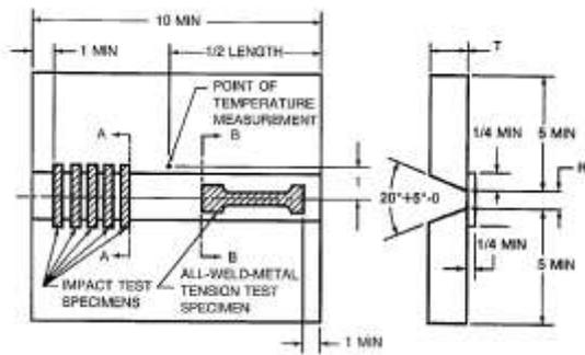
Figure 7. Plate for removal of specimens for tensile and impact test of the weld metal. (dimensions in inches). [2]
