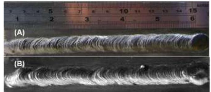
Figure 8. Visual appearance of the bead on plate weld deposited with impermeable electrode (A) and conventional E7018 electrode (B).
