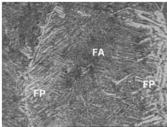
Figure 4 - Detail of the diagonal pattern region on Figure 3. Despite the Primary Ferrite (PF), common in this type of weld metal, it is possible to observe the presence of a large amount of Acicular Ferrite.
