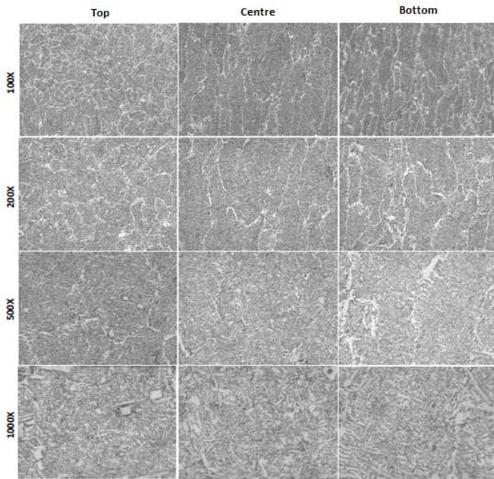
Figure 10 - Microstructure of the weld metal deposited with the impermeable electrode. Magnifications: 100, 200, 500 e 1000x.
