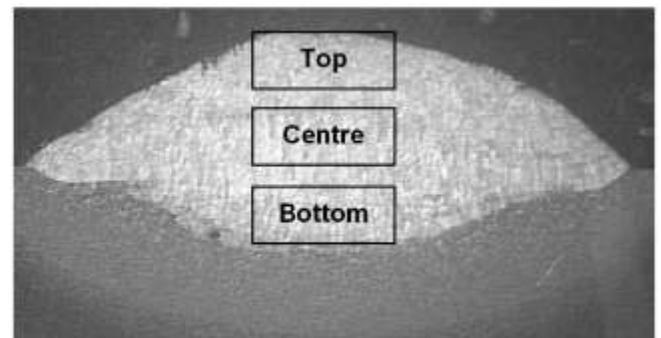
Figure 9 - Macrography of the weld metal
