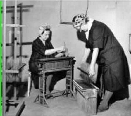
Figure 2 - Ladies coating the electrodes by immersion [1]
