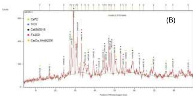
Figure 14 - diffraction patterns of the slag obtained in the welding with impermeable (A) and conventional (B) class E7018 electrodes.
