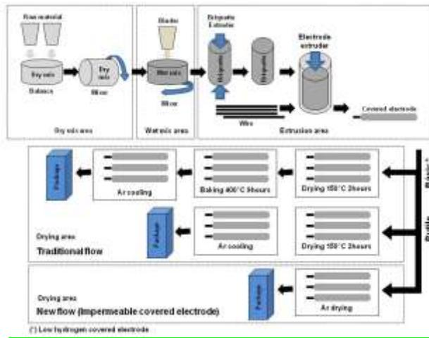
Figure 5 - Traditional and impermeable covered electrodes production flow chart
