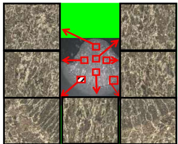
Figure 3 - Mosaic of underwater wet weld produced with an experimental E6013 electrode using polymer as binder. Depth: 0,5mm, polarity: DCEN; Electrode welding angle: 70°; welding current: 150 A; Chemical attach: Nital 2%; 100X.
