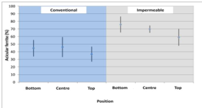
Figure 11 - Acicular ferrite content (Impermeable and conventional covered electrodes).
